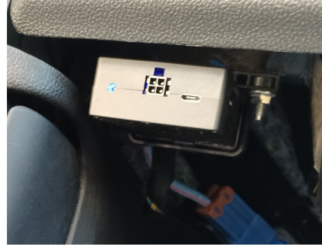
(b) The Freematics CAN data logger installed on OBD port of a vehicle
