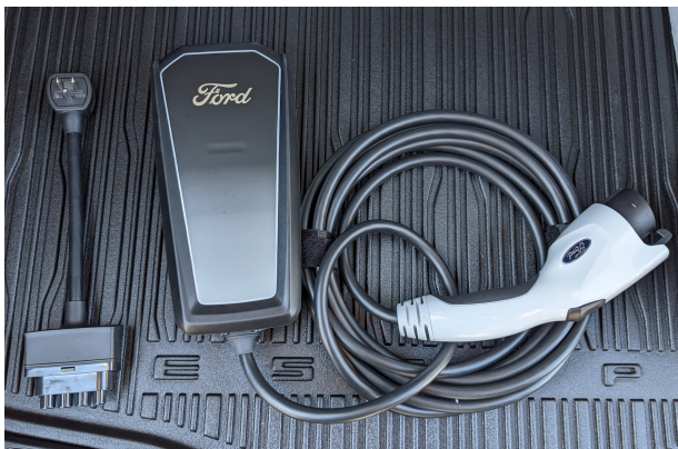
(b) Level 2 AC 220-volt charging port
