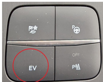
(a) Button for changing powertrain mode
