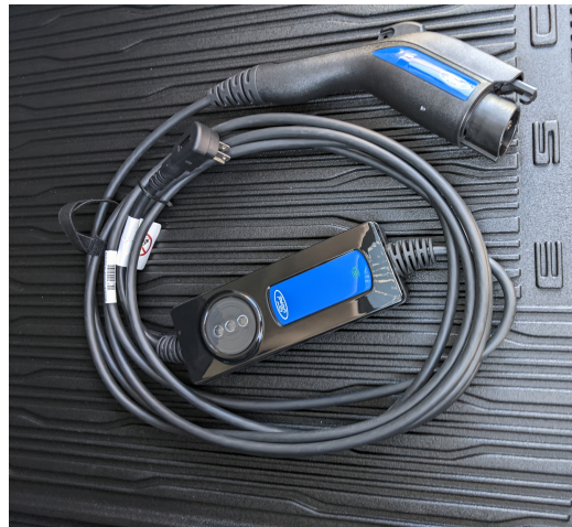
(a) Level 1 AC 110-volt charging port
